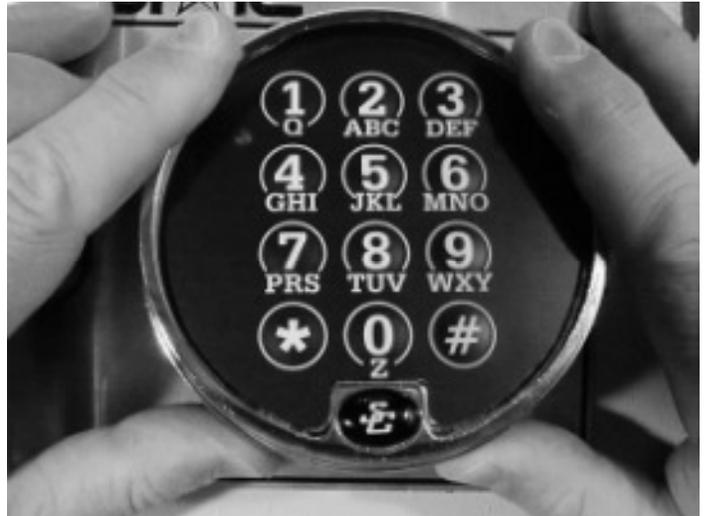
**STEP 2**—Turn the keypad over and remove both batteries. This is best done by grasping the bottom of a battery and pulling it gently away from the keypad circuit board. Do not use any type of tool to pry a battery from its holder.
